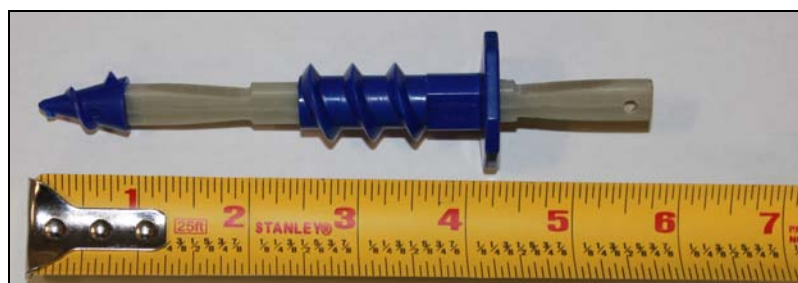
Figure 2-2: Square GFRP Anchor
