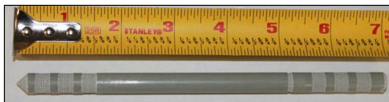
Figure 2-1: Cylindrical GFRP Anchor
