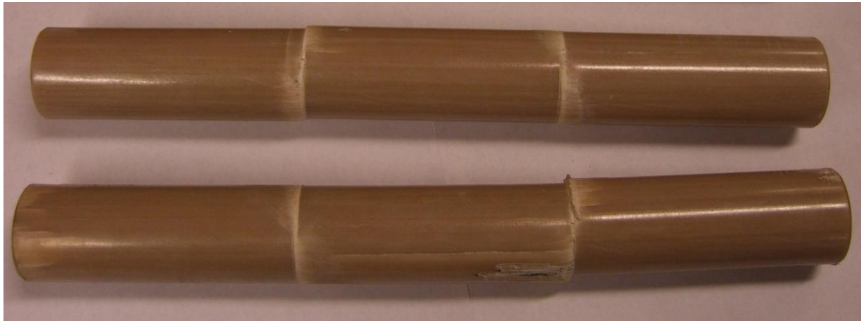
Figure 2: Initial Failure after short displacements
