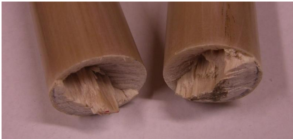
Figure 3: Secondary failure after large displacements
